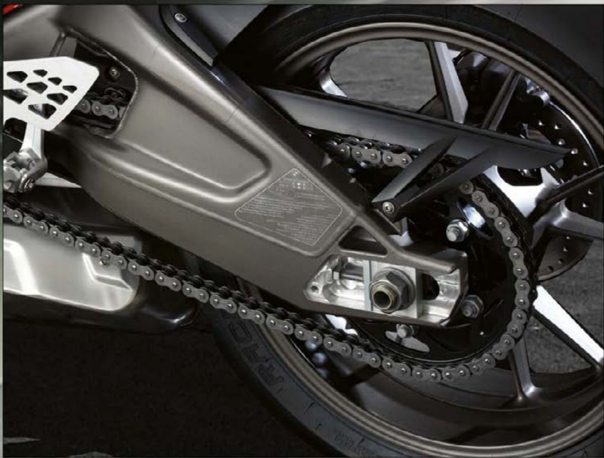
A long double swing-arm at the rear helps improve traction.
