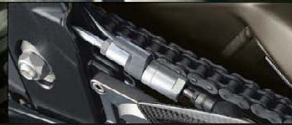
Change gear ten times faster, no declutching required: the optional HP gearshift assist.
