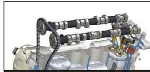
The 16 rocker arms are integral to the high revving of the RR engine.
